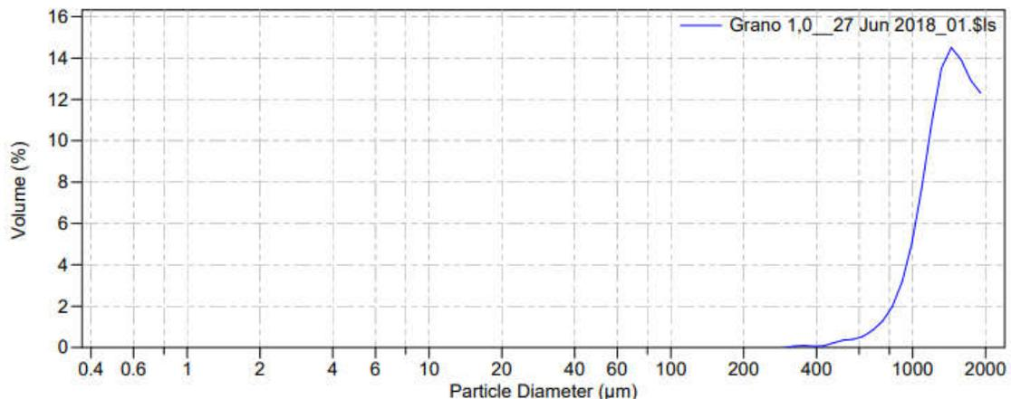
Figure 3-5 - Particle diameter distribution of grain sieved with 1.0 mm.
