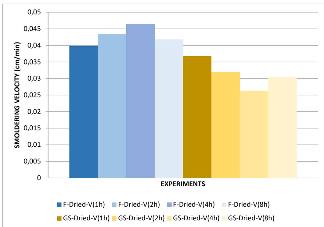
Figure 4-16 - Smoldering velocities for different ventilation times.
