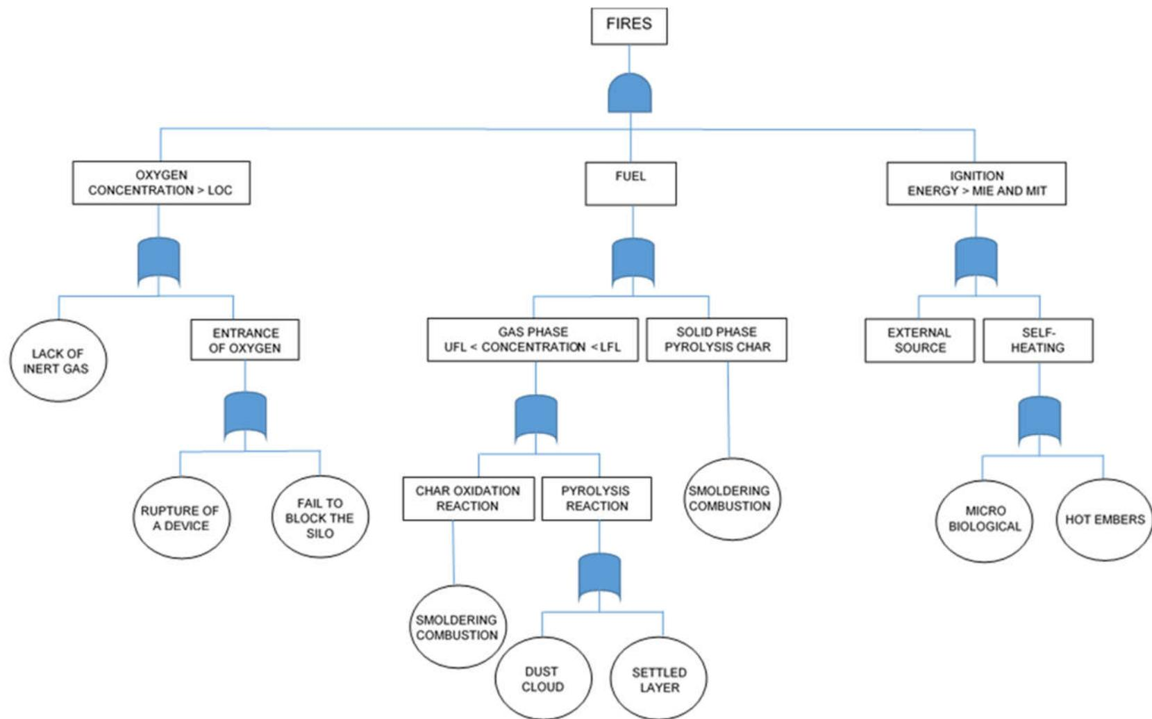
Figure 2-22 - FTA of fires in silos.
