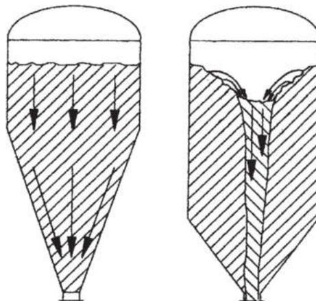
Figure 2-4 – Normal flow patterns: mass flow and funnel flow.
