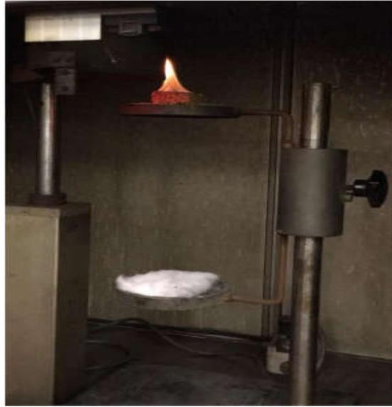
*Figure 3-8 - Experimental apparatus of Ignition time and extinguishability*
