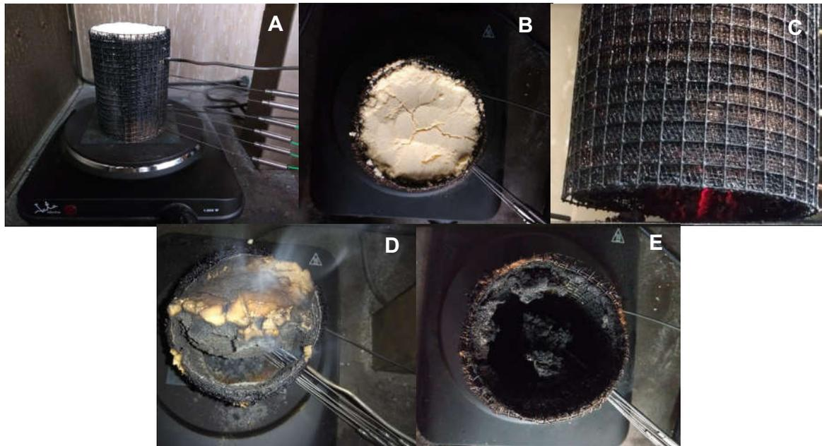
Figure 4-1 - Experiment sequence of dried corn flour without the ventilation system (F-Dried-NV).
