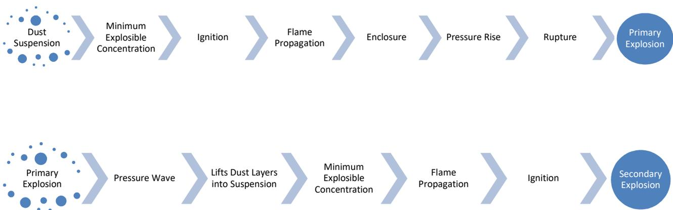
Figure 2-11 - Mechanism of Dust Explosions.
