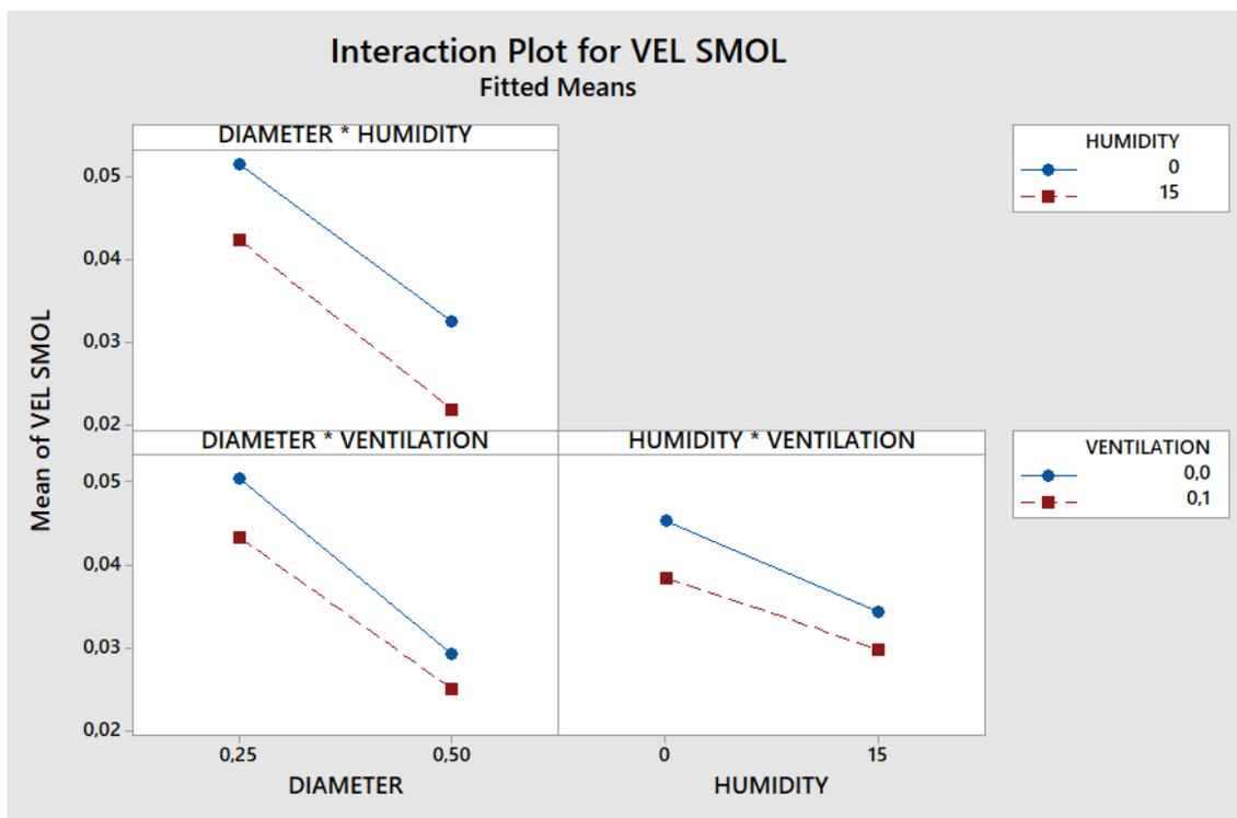
Figure 4-19 - Interaction plot for smoldering velocity.
