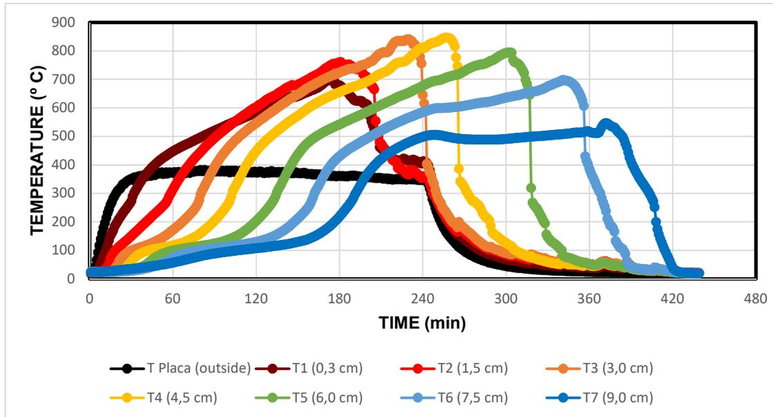
Figure B-1 - Dried corn flour without a ventilation system (F-Dried-NV\_2).
