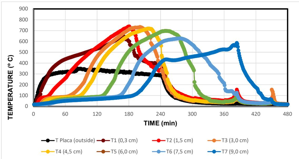
Figure B-4 - Wet corn flour without a ventilation system (F-Wet-NV\_2).
