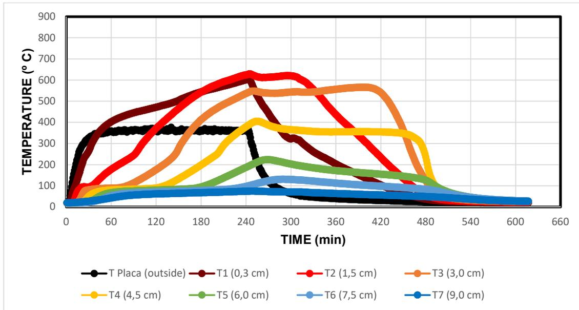
Figure B-13 - Wet grain 0.5 mm without a ventilation system (GS-Wet-NV\_3).
