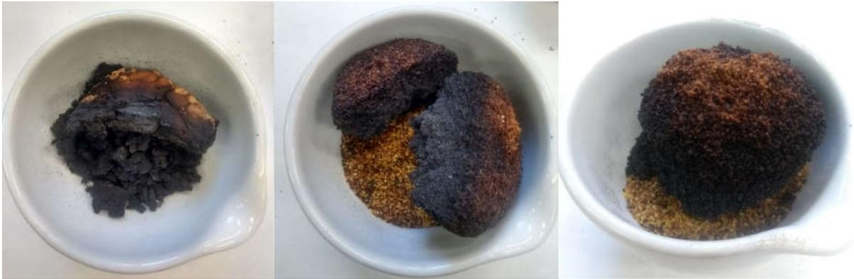
*Figure 4-2 - Residues of the three sizes of material used after the smoldering process: (F), (GS), (GL)*
