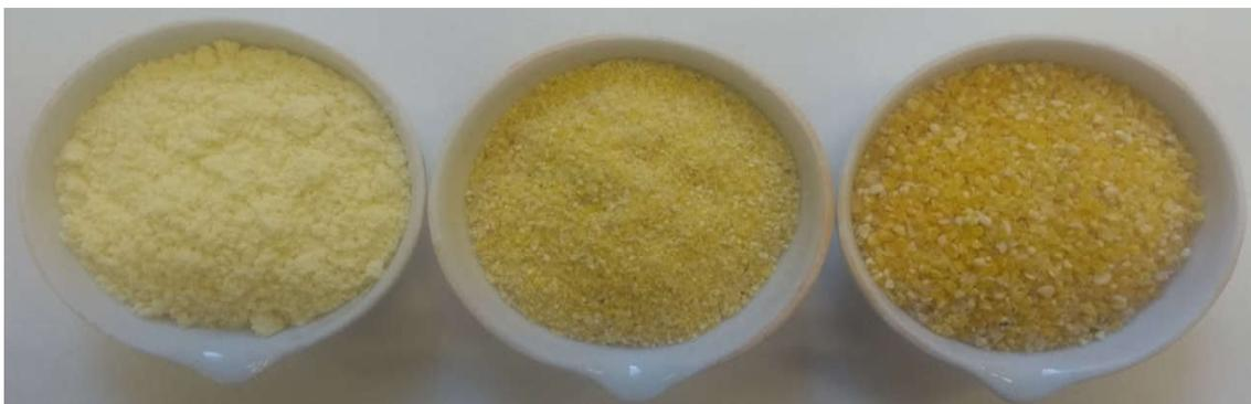
*Figure 3-2 – The three particle sizes of the experiments – corn flour, grain 0.5, and grain 1.0.*
