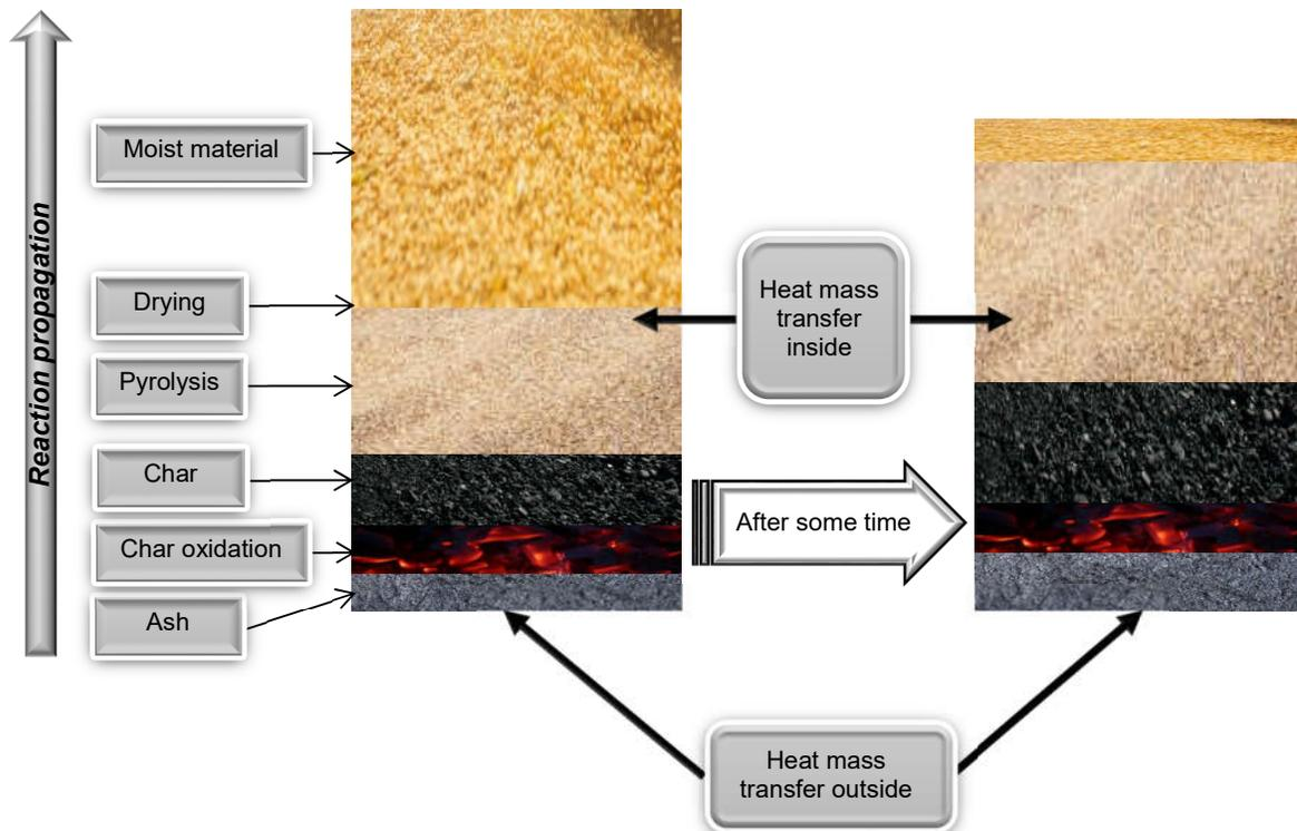
Figure 2-19 - Reaction Propagation.
