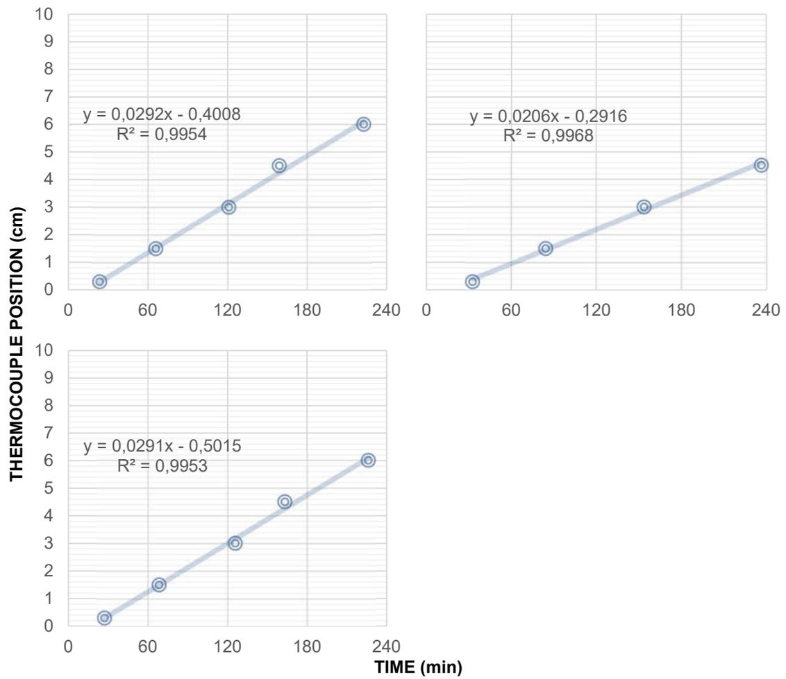
Figure C-6 - Dried grain (776.4  $\mu\text{m}$ ) with a ventilation system (GS-Dried-V) - sample 1, sample 2 and sample 3.
