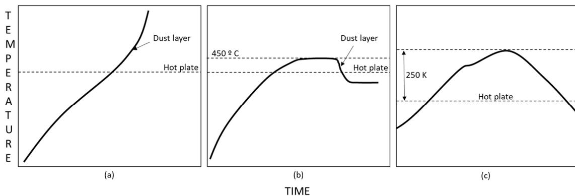
Figure 3-7 - Typical temperature-time curves for ignition of dust layer on the heated surface.
