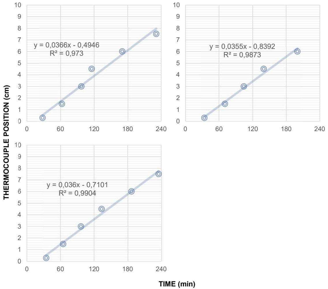
Figure C-5 - Dried grain (776.4 $\mu$ m) without the ventilation system (GS-Dried-NV) - sample 1, sample 2 and sample 3.
