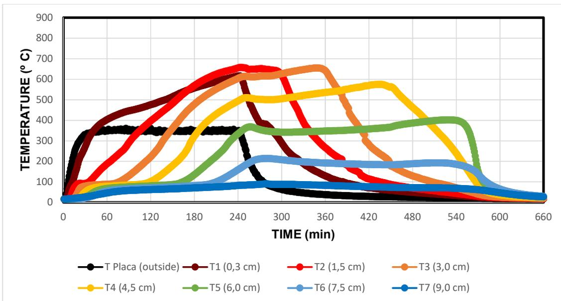
Figure B-12 - Wet grain 0.5 mm without a ventilation system (GS-Wet-NV\_1).
