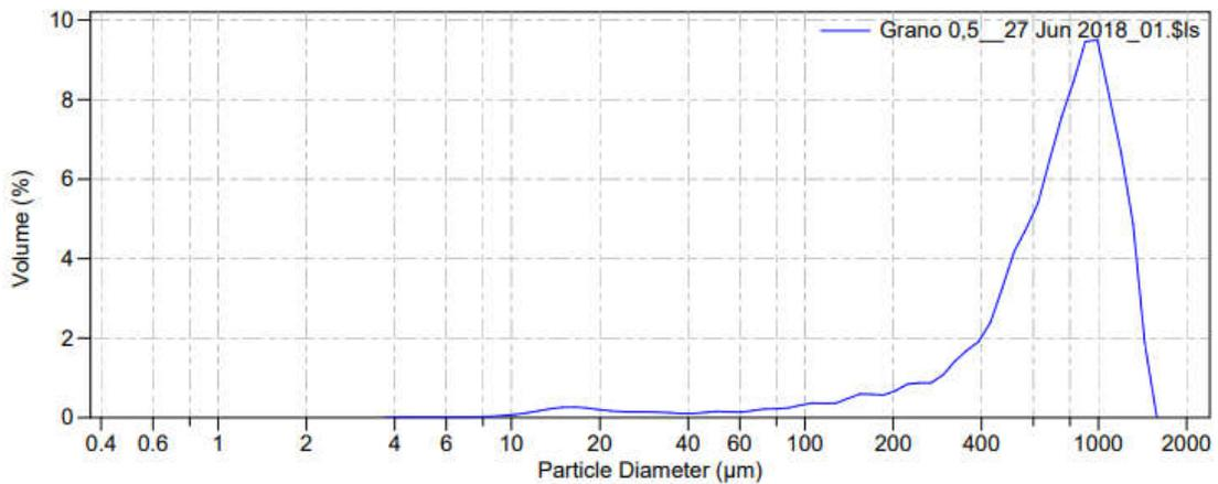
Figure 3-4 - Particle diameter distribution of grain sieved with 0.5 mm.
