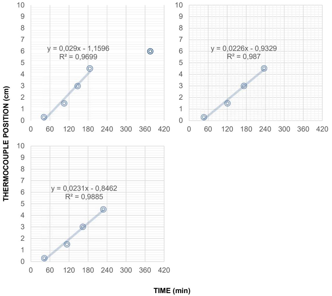
Figure C-7 - Wet grain (776.4  $\mu\text{m}$ ) without the system ventilation (GS-Wet-NV) - sample 1, sample 2, and sample 3.
