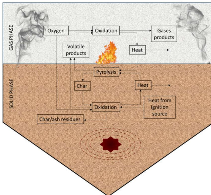
Figure 2-21 - Process diagram of reactions in silos.
