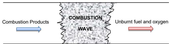
Figure 2-3 - Structure of a combustion wave.
