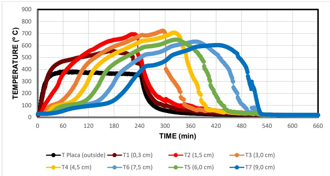
Figure B-17 - Dried cornflour with a 2h ventilation system (F-Dried-V(2h)\_1).
