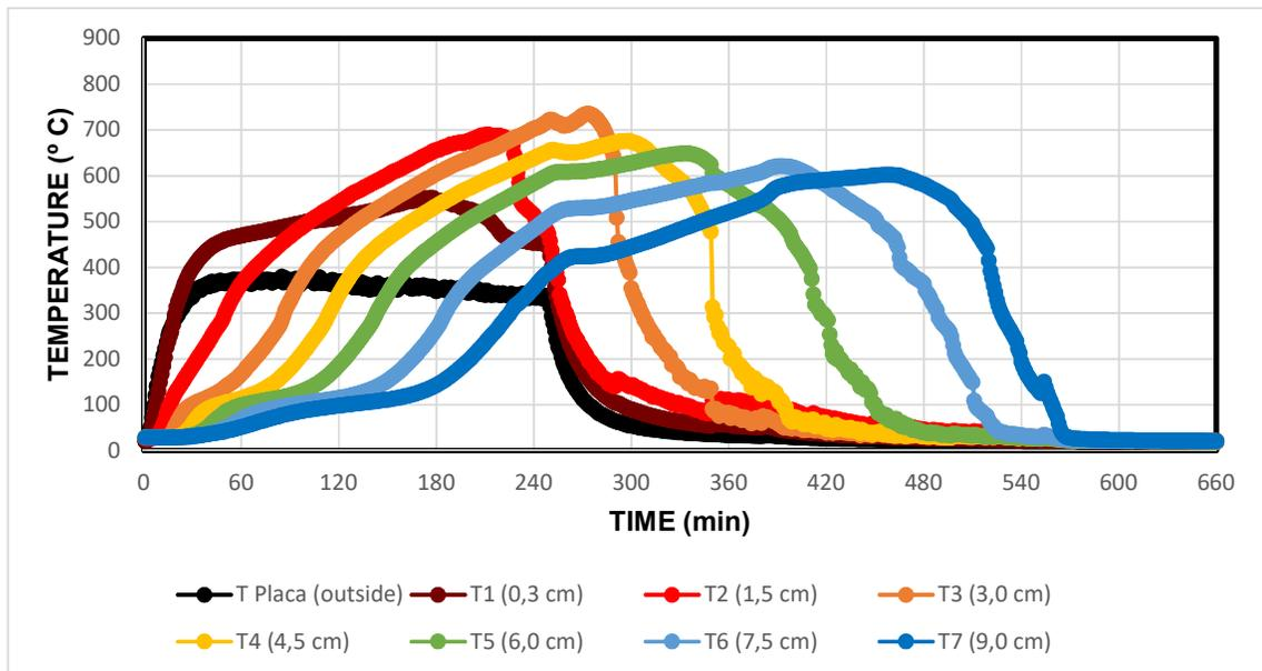
Figure B-18 - Dried corn flour with an 8h ventilation system (F-Dried-V(8h)\_1).
