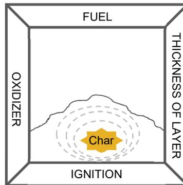
Figure 2-20 - Square of smoldering combustion.
