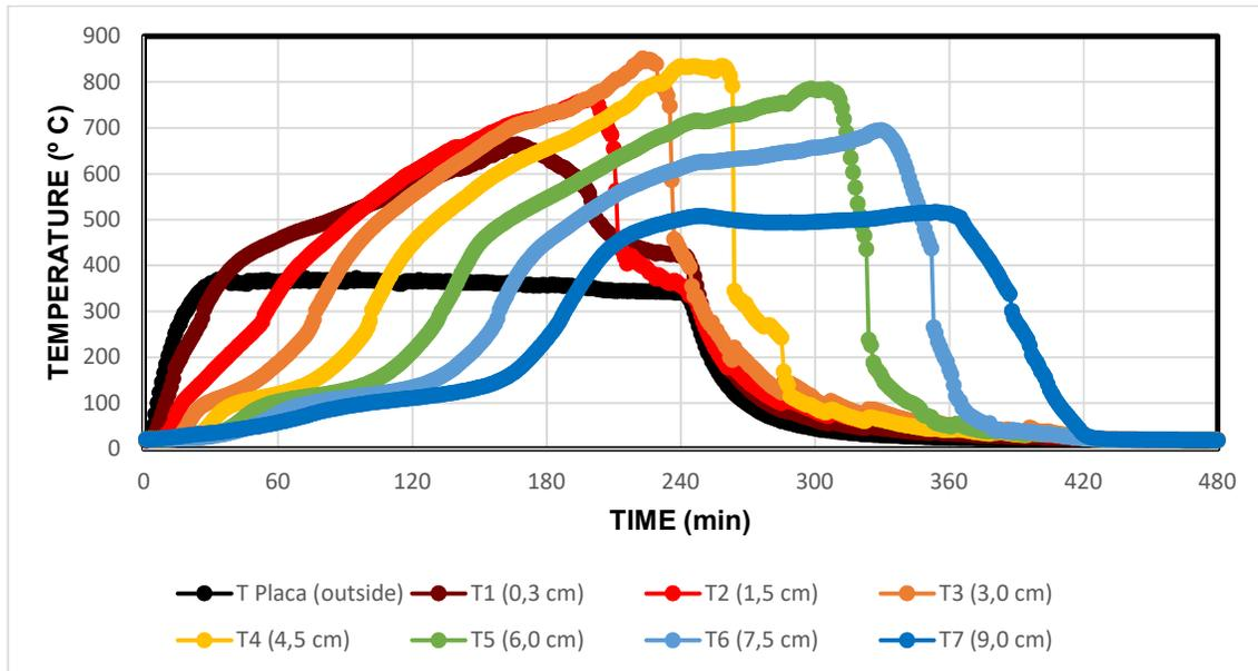
Figure 4-3 - Dried corn flour without a ventilation system (F-Dried-NV\_1).
