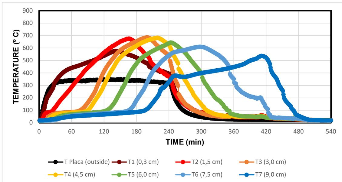
Figure 4-5 - Wet corn flour without a ventilation system (F-Wet-NV\_1).
