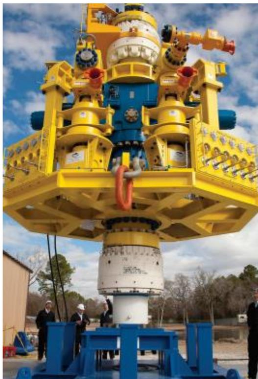
Figura 13: *Capping Stack*
