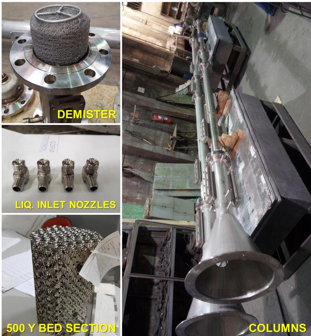
**Figure I.6. PCAPP Columns and their internals**
