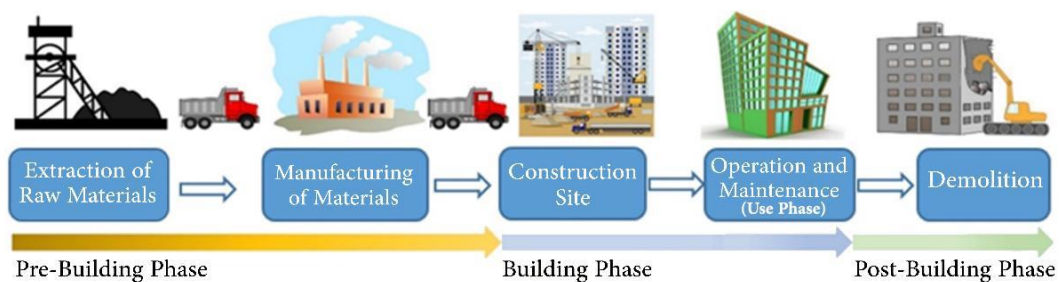
Figure1. Life cycle building phase
